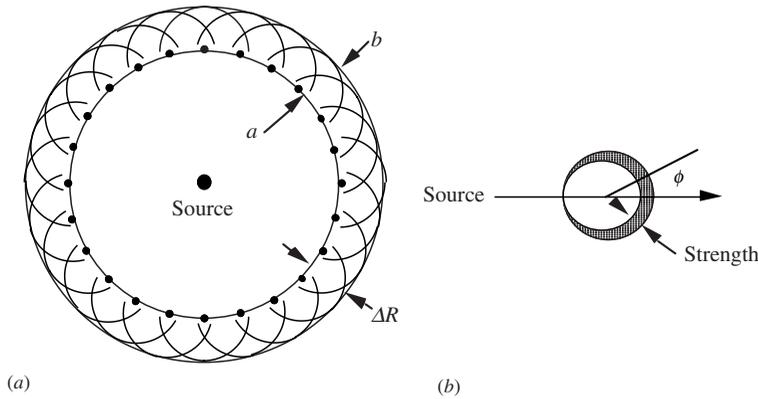
**Fig. 1.3.** Huygens wavelet construction for a pulse. (a) Points on a previous pulse wave front at “a” are the sources of wavelets whose envelope becomes the new wave front, “b.” The wave front thereby moves from a to b. (b) The dependence of wavelet strength on propagation direction, is shown by shadowing. The analytical description of the dependence on  $\phi$ , (1.4) is called the Stokes obliquity factor.
