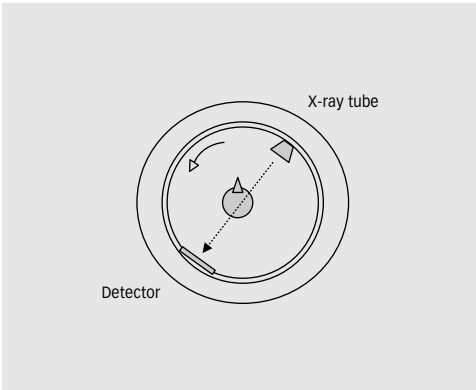
Fig. 1.14. Diagram of a typical CT scanner. The patient is placed on the couch and the X-ray tube rotates 360° around the patient, producing pulses of radiation that pass through the patient. The detectors rotate with the tube, on the other side of the patient detect the attenuated X-ray pulse. This data is sent to a computer for reconstruction.
