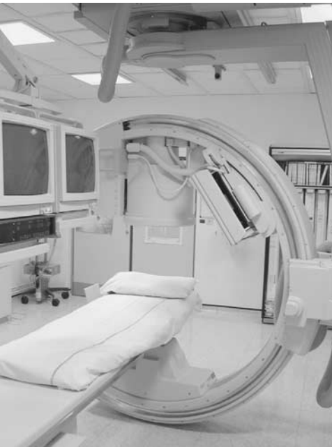
Fig. 1.1. An example of a fluoroscopy machine that uses X-radiation to produce images of patients. The tube can be rotated around the patient to provide views from different projections. Moving images can be viewed using the image intensifier or static images can be obtained.
