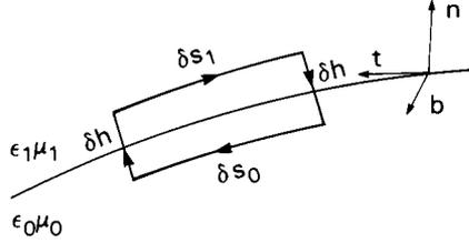
Fig. 1.5.2 Loop at the interface between two media. The vectors  $\mathbf{n}$ ,  $\mathbf{t}$ , and  $\mathbf{b}$  indicate the directions normal to the interface surface, tangential to the surface, but in the plane of the loop, and the orthogonal direction, also tangential to the interface, but normal to the loop area.
