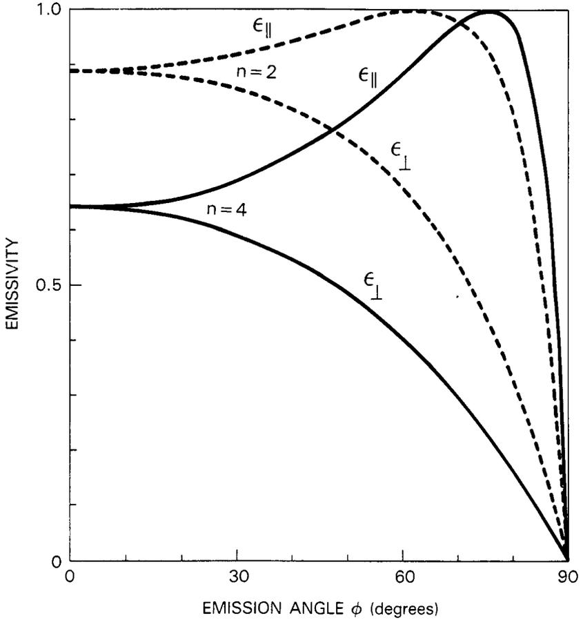
Fig. 1.6.1 Emissivity of a smooth flat surface with an index of refraction,  $n$ , as a function of emission angle. Both planes of polarization are shown for  $n$  equal to 2 (dashed lines) and 4 (solid lines).
