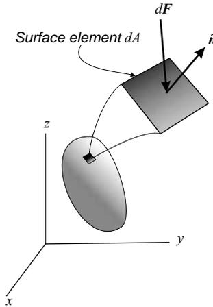
Figure 1.5. Traction vector acting on a surface element.
