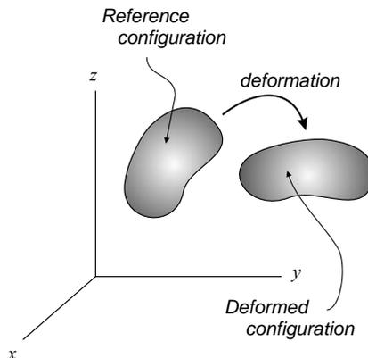
Figure 1.2. Reference and deformed configurations of body.
