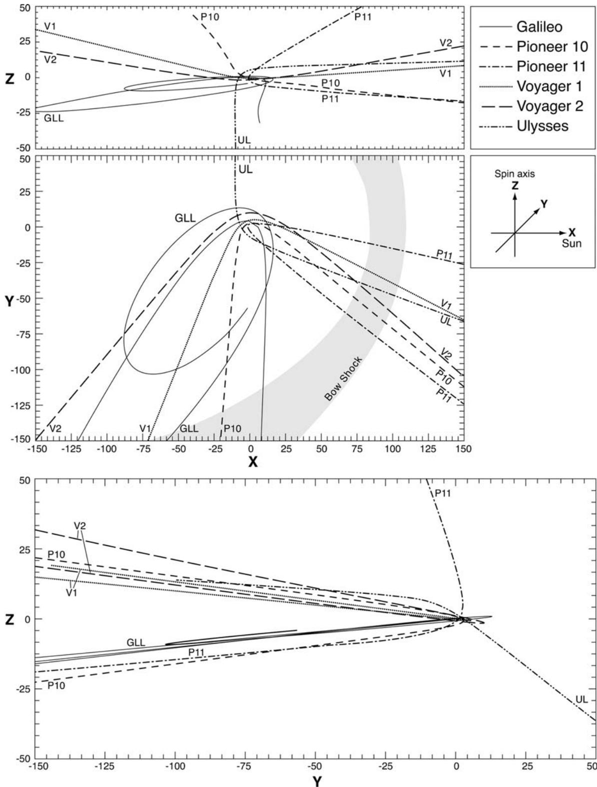
**Figure 1.1.** Trajectories of the five spacecraft flybys and the first orbit by *Galileo*. The co-ordinate system is centered on Jupiter and has the  $x$  axis pointed towards the Sun, the  $z$  axis is pointed along Jupiter's spin axis and the  $y$  axis makes a right-handed set (and points towards Jupiter's dusk side). The units are in jovian radii. (Courtesy of S. Joy, UCLA.)
