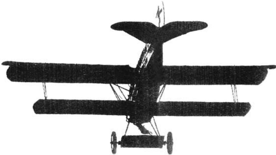
**Figure 1.5** The Fokker D-VII, built without wing dihedral, showing no concern for spiral stability. This machine had horn aerodynamic balances at the tips of all control surfaces, to reduce control forces. (From *Progress in Airplane Design Since 1903*, NASA Publication L-9866, 1974.)
