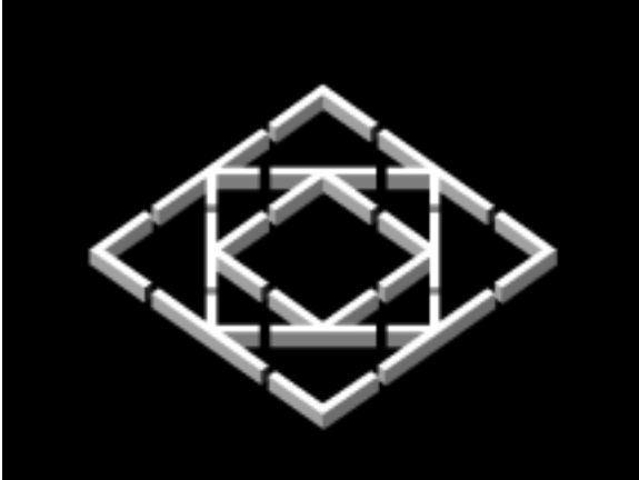
Figure 1.19. Roriczer's shape developed as an assembly of K-shaped and L-shaped precast concrete elements.
