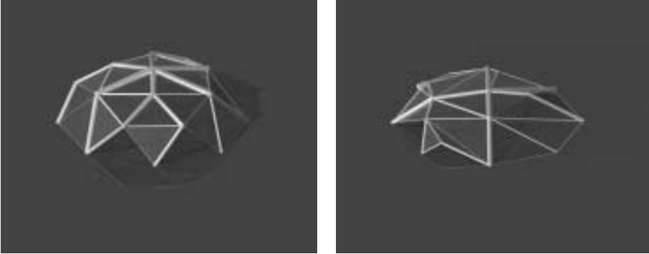
Figure 1.8. Unusual dome designs generated by Shea's shape annealing procedure.
