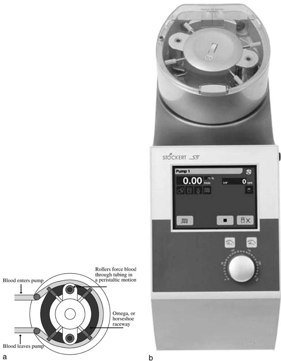
Figure 1.5. (a) Line drawing of a roller pump; (b) a roller pump. (Reproduced with kind permission from Sorin Group.)
