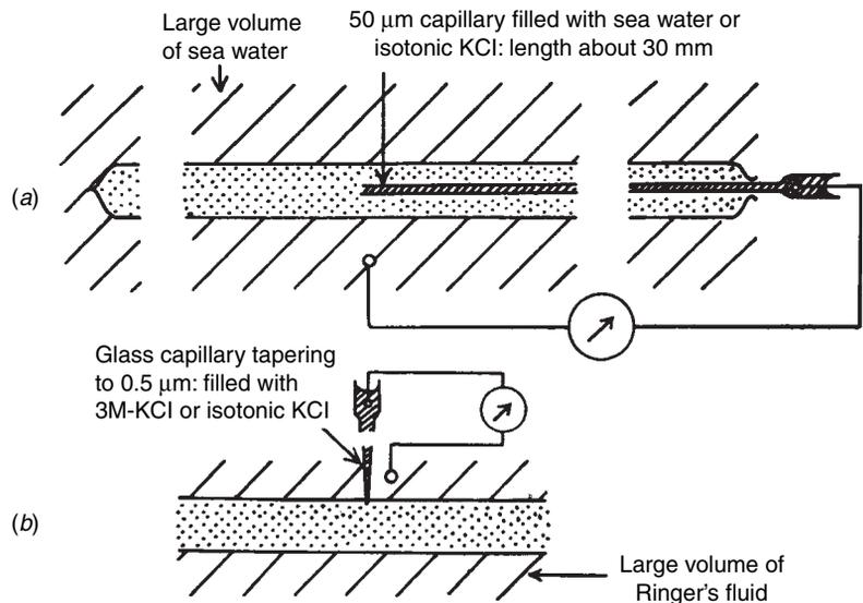
microelectrode is then filled with 3 M KCl, and an Ag/AgCl electrode is inserted at the wide end. With various refinements, microelectrodes of this type have been used for direct measurement of the membrane potential not only in single neurons, but also in many other types of cell.
