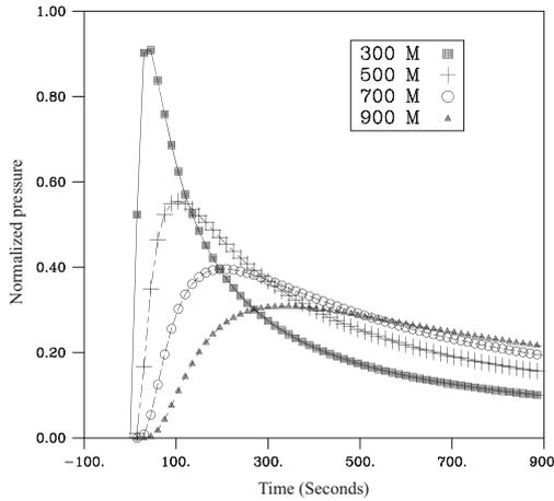
Figure 1.5 Pressure variation  $p(r, t) = \frac{C}{\sqrt{t^3}} \exp\left(-\frac{1}{4D} \frac{r^2}{t}\right)$ , associated with an impulsive source corresponding to four observation points located at successively greater distances from the source.
