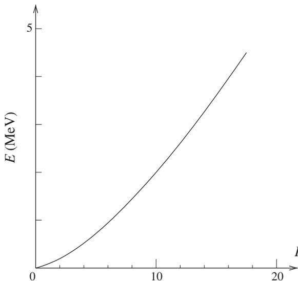
Figure 1.4. Schematic representation of the (discrete) energy levels of the (ground state) rotational band of a quadrupole deformed atomic nucleus as a function of the angular momentum  $I$  ( $E = (\hbar^2/2\mathcal{I})I(I + 1)$ , where  $\mathcal{I}$  is the moment of inertia).
