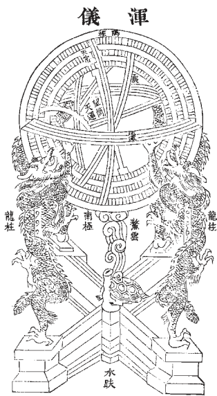
The hun yi (armillary sphere), one of the major astronomical instruments in ancient China. This sketch of the hun yi is by Su Song of the Song Dynasty.
