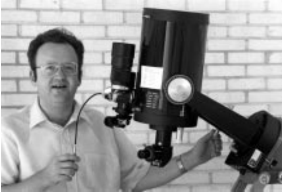
Figure 1.2 The author gets ready to photograph star fields with a camera and 180-mm lens mounted “piggy-back” on a 20-cm (8-inch) Schmidt-Cassegrain telescope. (Melody Covington)
