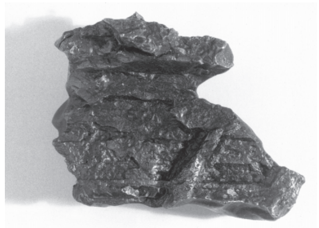
Fig. 3.5. These two photos show front and back sides of a Sikhote-Alin iron meteorite. The left image shows an ablated smooth surface with extensive pitting. The right image shows the opposing side where fragmentation took place near the end of the ablation period revealing parallel-running linear features typical of octahedrite meteorites. The specimen measures 11.8 × 9.5 cm. (Specimen provided by Dr David Mouat, Desert Research Institute, University of Nevada System. Photos by O. Richard Norton.)
